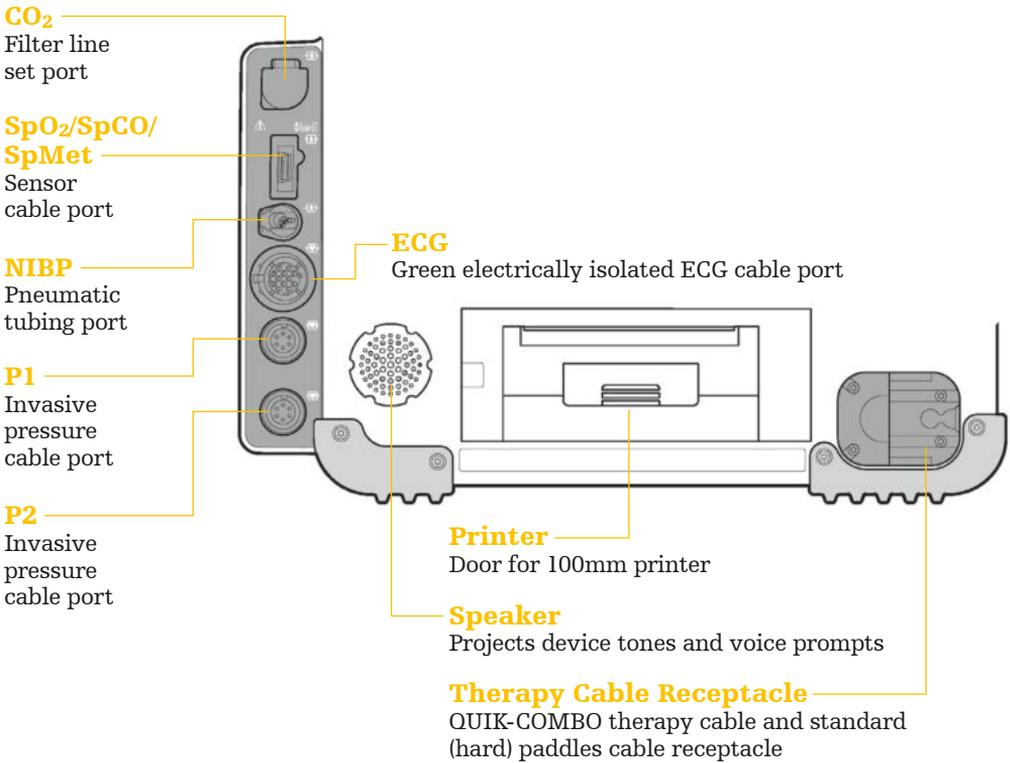
**Note:** If your LIFEPAK 15 monitor/defibrillator is configured for temperature monitoring, P1 and P2 are replaced by a single port labeled TEMP.
